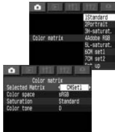
The EOS-1D Mark II has five pre-set color matrixes, the same as the EOS-1D and the EOS-1Ds. The matrixes have been re-tuned to control red saturation. The Mark II adds two additional matrixes which can be user-set for color space (sRGB or Adobe RGB), color density (5 levels) and color hue (5 levels). Color matrix settings on the menu now state what each setting is (standard, portrait, high-saturation, Adobe RGB, low-saturation) rather than just a number.
