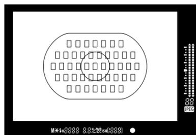
The 45-point AF unit is the same as the EOS-1D's. However, the AF-related circuitry and the AF algorithm incorporate a completely new design so that the AF performance surpasses that of the 1D. The EOS-1D had a single CPU for AF operations from focus detection to
